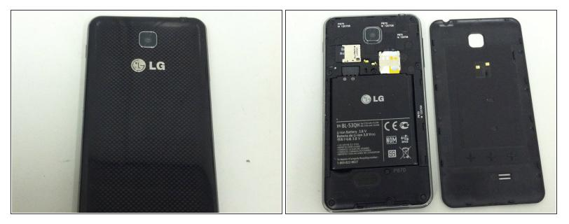
• Turn the device over and pull the back plastic cover off by inserting your fingernail into the opening at the bottom of the phone and gently pulling.
