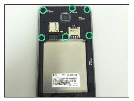
Remove the remaining 6 screws securing the plastic frame to the back housing
