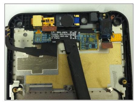
Peel off the adhesive portion of the LCD ribbon cable from the back of the phone
