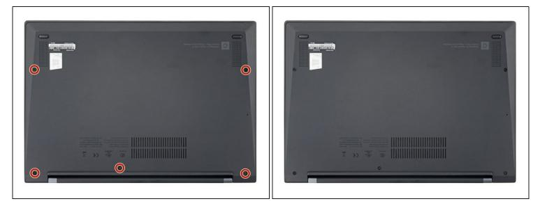
A For your safety, discharge the battery below 25% and power down your device before disassembly.
