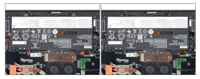
• Use a Phillips #1 screwdriver to remove the six 4.9 mm screws securing the battery to the laptop chassis.
