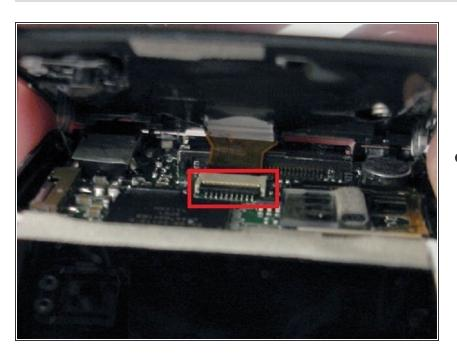
Remove ribbon cable connect to the face plate. Lift the face off and flip the brown ribbon release flap on the connection on the board. (The flap in this picture is black, opposite the cable. Lift the edge that is closest to you in the picture in order to release the cable.)
