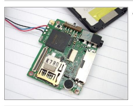
Remove the board by lifting on the left side first as to work around the on off switch.
