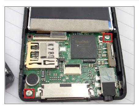
Remove two (in some versions there are 3) screws holding the board down
