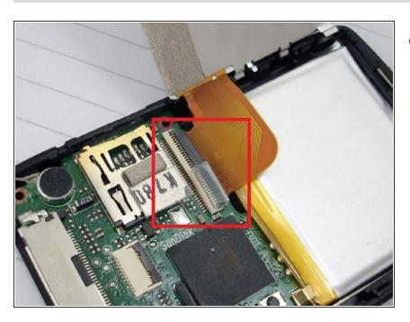
Carefully flip the LCD over and disconnect the LCD cable from the board
