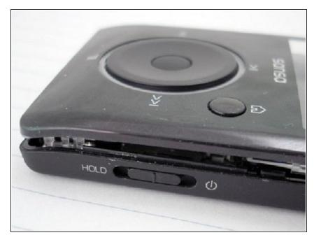
Pry open and pop the clips. Note that the bottom two clips are held in with a little bit of rubbery glue. Don't rip the face off too quick since there is a ribbon cable you need to disconnect.
