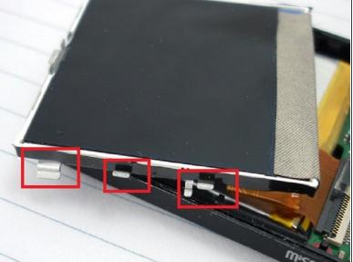
Remove LCD by releasing the 4 clips on each side of the LCD, be carefully to not damage the LCD
