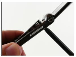
Rest the spudger/scewdriver between the top of the black plastic and the metal body of the phone and leaver the two apart to release the top clip on the keyboard.and the top of the keypad pops out from the RAZR2.
