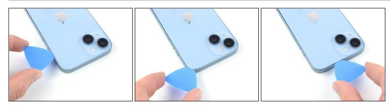
• Insert your pick underneath the top right edge of the phone. Slide it around the topright corner and halfway across the top edge.
