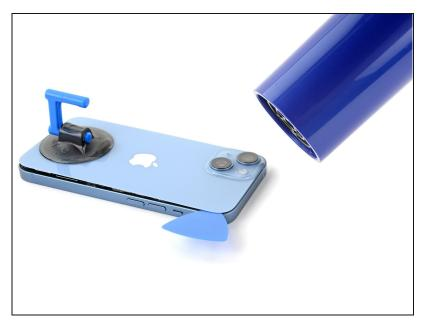
• Use a hair dryer to heat the top edge of the iPhone for 90 seconds or until the rear glass is slightly too hot to touch.
