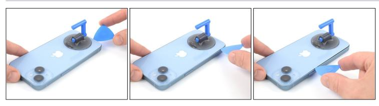
• Slide the opening pick around the lower left corner and up the left edge of the iPhone, slicing through the adhesive holding the rear glass in place.
