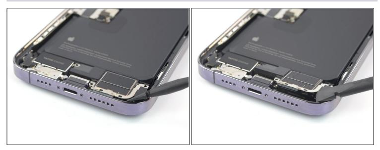
• Use the flat end of a spudger to pry up and loosen the loudspeaker from the bottom right corner of the phone.
