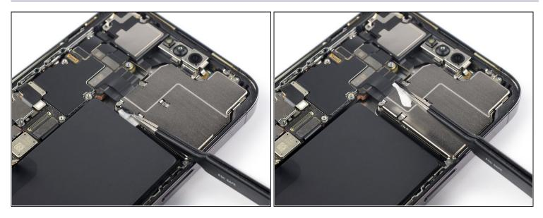
• Pull the remaining adhesive tab using the same procedure. Try not to snag the adhesive on anything.
