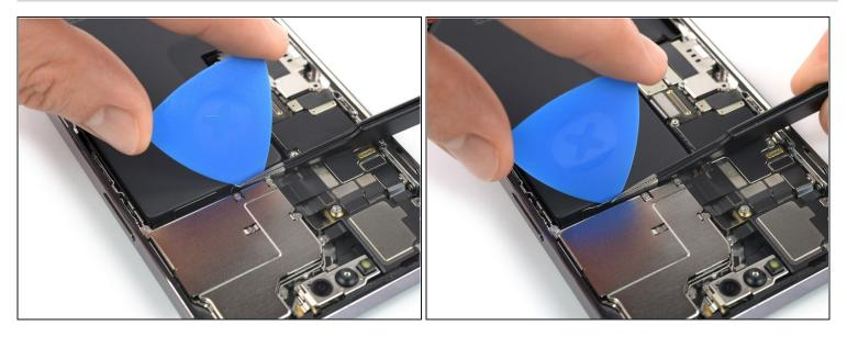
• Use a pair of blunt-nosed tweezers and an opening pick to peel up the two remaining battery adhesive pull-tabs from the top edge of the battery.
