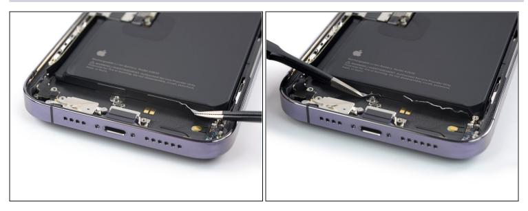
▲ **Caution:** Don't jab the battery with any sharp tools. A punctured battery may leak dangerous chemicals or catch fire.
