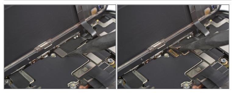
• Use the pointed end of a spudger to disconnect the second display cable by prying the connector straight up from its socket.
