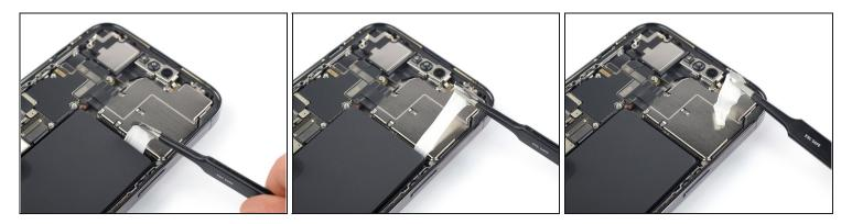
• Using the same procedure as before, pull the third tab from underneath the battery. Try not to snag the adhesive on anything.
