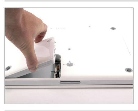
• Lift the battery out of the computer.
