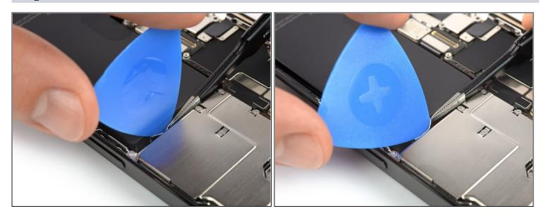
• Use a pair of blunt-nosed tweezers and an opening pick to peel up the remaining battery adhesive pull-tab from the top edge of the battery.
