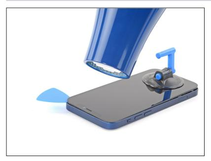
Use a hair dryer to heat the top edge of the iPhone for 90 seconds or until the screen is slightly too hot to touch.
