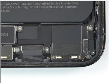
Use a Phillips driver to remove the four 1.5 mm-long screws securing the loudspeaker.
