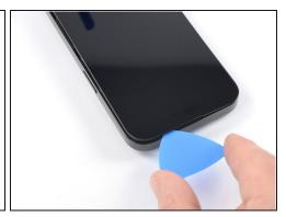
Slide the opening pick around the top right corner of the iPhone to separate the top adhesive.
