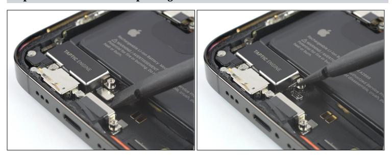
• Use a spudger to disconnect the Taptic Engine by prying the connector straight up from its socket.
