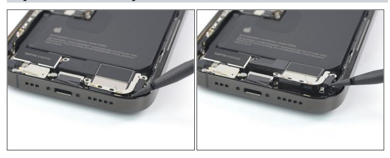
• Use the flat end of a spudger to pry up and loosen the loudspeaker from the bottomright corner of the phone.
