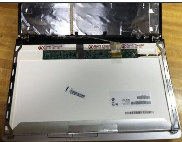
Grab the top corners of the LCD and gently fold the LCD down until it is resting on the keyboard.
