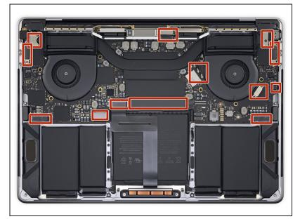
⚠ Carefully lift up the logic board, make sure none of the connectors are connected, also make sure they aren't caught on the logic board.
