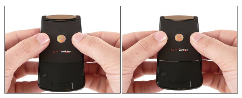
Push the rear cover toward the hinge of the RAZR2. The panel will slide about 3 mm.
