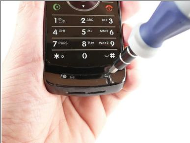
Remove the two 4-mm T5 Torx screws, previously hidden beneath the flip stop bumper pad.
