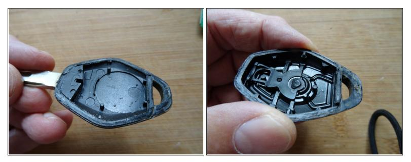
• Here is what the inside of the casing looks like. The circuit board has already been removed.
