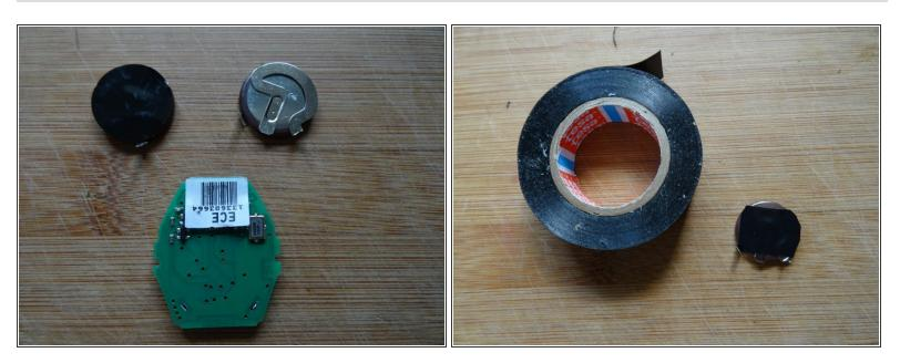
• If there isn't an insulation layer on the back, then place a piece of insulation tape there.
