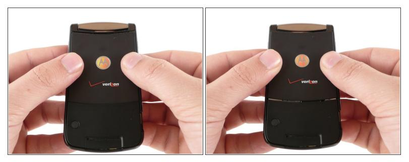
• Push the rear cover toward the hinge of the RAZR2. The panel will slide about 3 mm.
