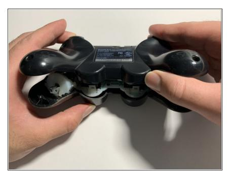
Remove the back shell from the controller by pulling the front and back shells apart at the same time.
