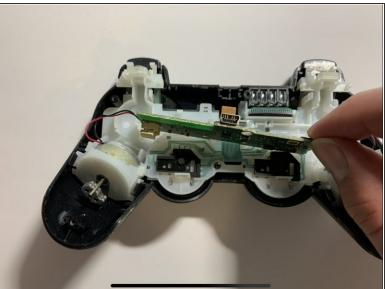
Remove the motherboard by pushing the two white hooks on both the left and right side of the motherboard backwards.
