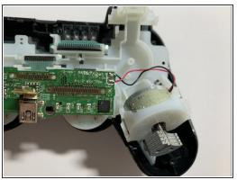
To remove the white body piece, start by using your fingers to unhook the small black hooks securing the left and right rumble motors.
