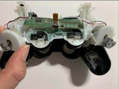
Remove the white body piece from the controller by pushing the unhooked left and right rumble motors in an upward direction.
