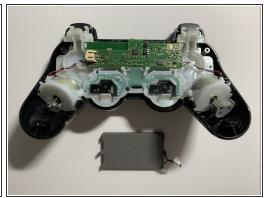
Disconnect the battery from the controller by pressing the two sides of the connector and pulling it out.
