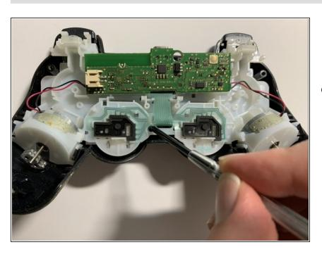
Use a Phillips #1 screwdriver to remove the single 7.2 mm screw, which secures the white body piece inside the controller.
