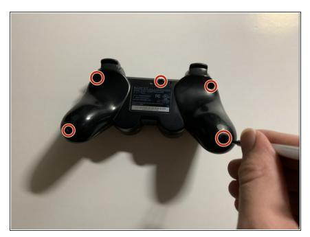
Use a Phillips #1 screwdriver to remove the five 7.2 mm Phillips screws which hold the back shell to the controller.
