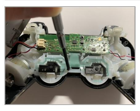
Use the Phillips #1 screwdriver to screw the single 7.2 mm Phillips screw to secure the white body piece inside the controller.
