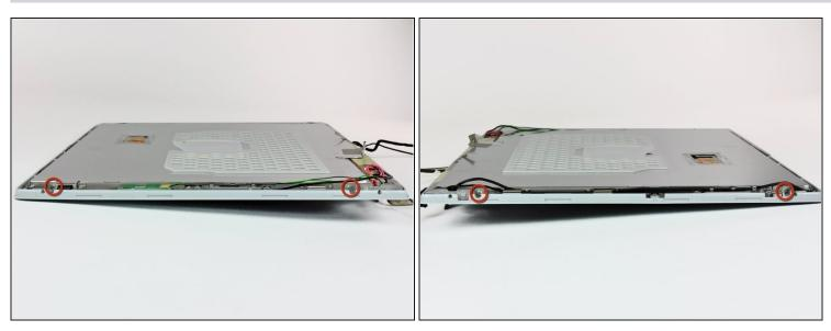
• Remove the two Phillips screws securing each side of the LCD to the clutch hinge frame (four screws total).
