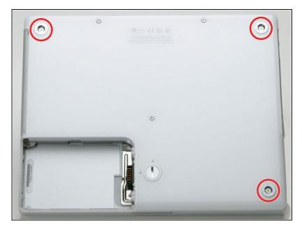
Remove the three 5.2 mm newly-revealed Phillips screws.
