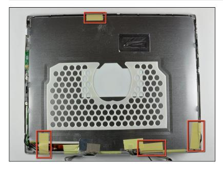
Remove the pieces of readily removable tape from around the perimeter of the display.
