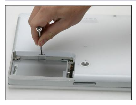
There is a slot on the wall of the battery compartment that locks the lower case in place.
