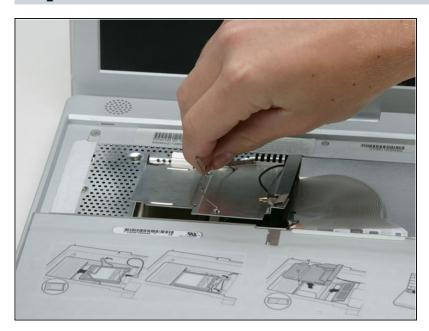
Grasp the metal bracket on top of the RAM shield and pull upward to remove the shield.
