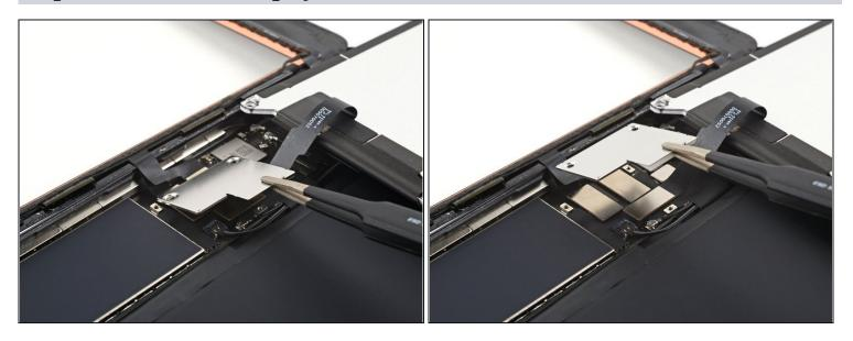
• Remove the display cable bracket.
