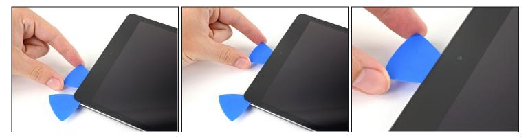
• Slide the opening pick along the top edge of the iPad, stopping just before you reach the front camera.
