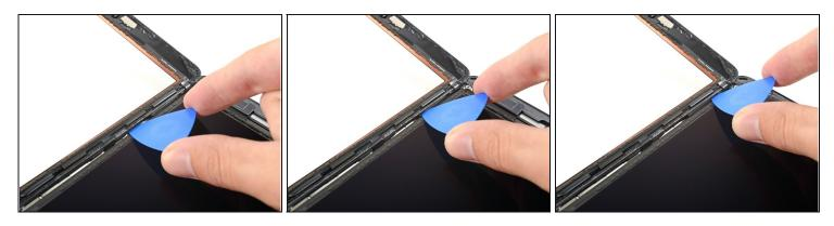
• While supporting the digitizer, slide an opening pick between the two digitizer cables to separate the last of the adhesive.
