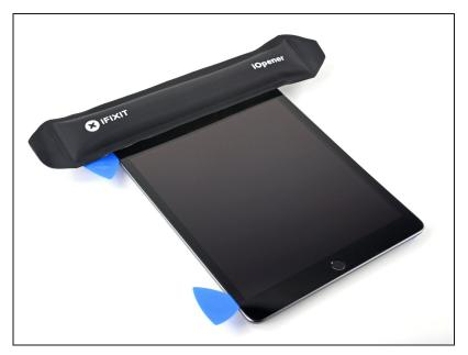
Heat an iOpener and apply it to the top edge of the iPad for two minutes.
