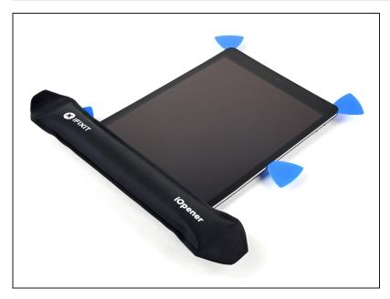
Heat an iOpener and apply it to the bottom edge of the iPad for two minutes.
