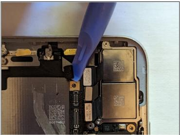
• Disconnect the WiFi Antenna cable connector.
