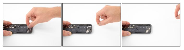
Repeat the previous step to remove the strip on the opposite side, leaving the center strip for last.
