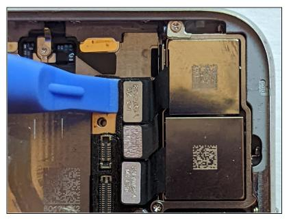
• Disconnect the Wide-Angle Camera cable connector.
