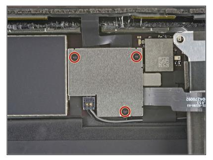
Use a Phillips screwdriver to remove the three 1.4 mm-long screws securing the display cable bracket.
