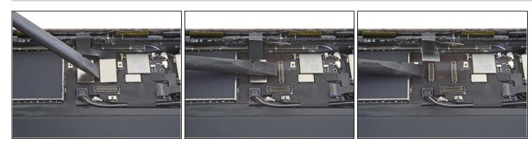
• Use the flat end of a spudger to disconnect the two digitizer cables by lifting straight up on the press connectors.
