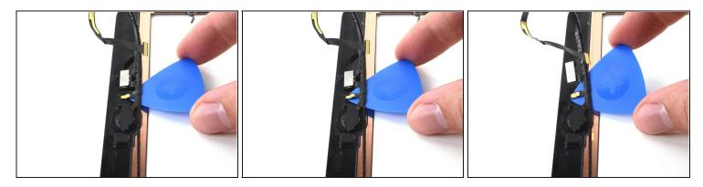
• Slide an opening pick under the top of the home button cable to loosen the metal contact off of the home button bracket.
