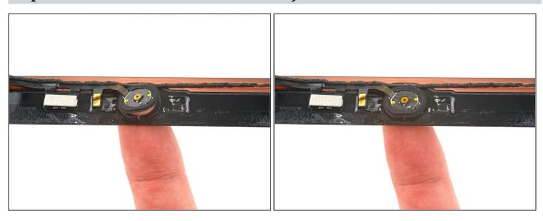
• Use your finger to push the home button through the front of the front panel to separate the adhesive holding it in place.
