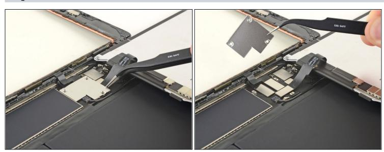
• Remove the display cable bracket.
