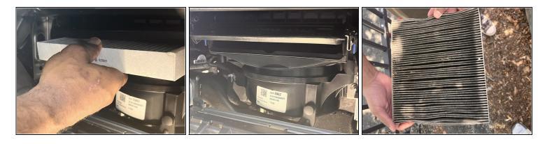
Remove the filter, and check for debris in the filter box.
