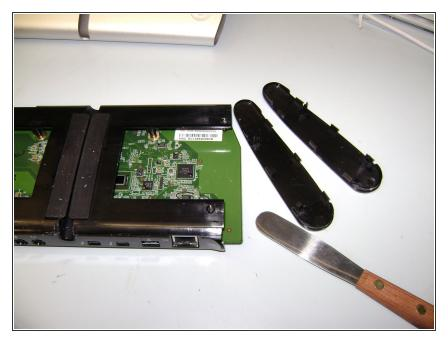
• The next step is to use the putty knife to pry off one of the two plastic endcaps, they snap out and the circuit board slides out.
