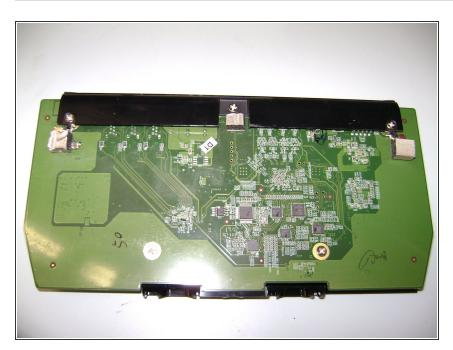
• Use the phillips screwdriver to remove 5 more screws to remove the plastic mounting frame.
