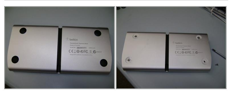
Use a putty knife to remove the four rubber feet. Once removed, there are 4 phillips screws to be removed.
