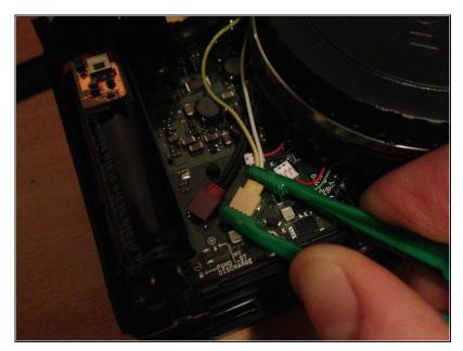
Reattach the red and yellow connectors on the front of the camera. Be sure to route the cables so they cannot interfere with the front cover when replaced.
