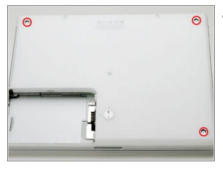
Remove the three newly-revealed Phillips screws.
