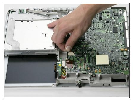
Remove the yellow tape securing the DC cable to the metal framework and disconnect the DC cable from the logic board.
