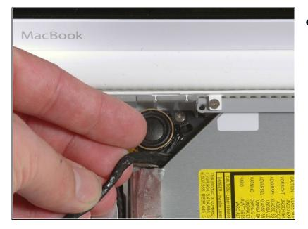
Pull up the display data cable from along the edge of the optical drive to reveal a silver Phillips screw.
