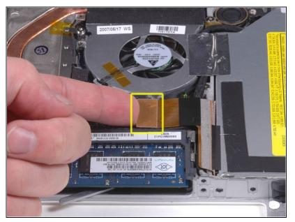
• Disconnect the orange optical drive ribbon cable connector from the logic board by prying it straight up using either a finger or a spudger.
