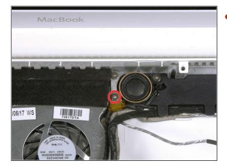
If you didn't remove the ground lug retaining screw in step 20 above, remove it now.
