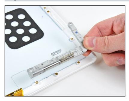
• Lift the right clutch hinge out of the rear display bezel.
