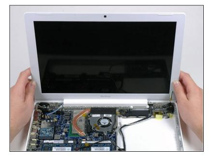
• Grasp the display assembly on either side and lift it up and out of the computer, taking care that the cables attached to the display don't snag on parts in the lower case.
