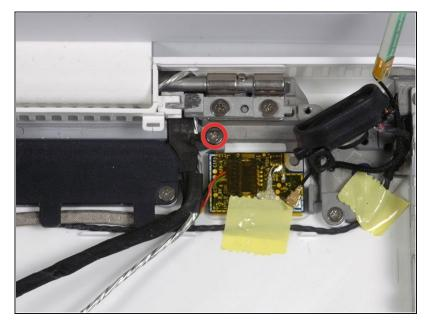
Remove the single 3 mm Phillips screw securing the ground lug in the display data cable located just above the Bluetooth board. This screw may also be securing a ground lug in the speaker cable.
