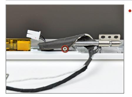
Remove the single 3.2 mm Phillips screw securing the display data cable to the right clutch hinge.
