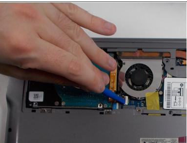
Using the plastic opening tool, push the hard drive connector clip upwards in order to release the cable.
