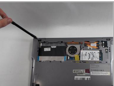
Remove the two 4 mm Phillips #00 screws formerly concealed by the pads.
