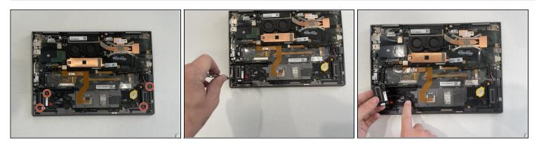
• Use a Phillips #1 screwdriver to remove the four 1.8 mm screws.
