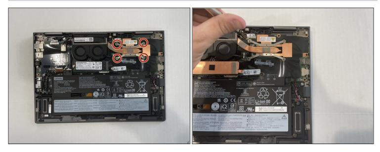
Use a Phillips #000 screwdriver to loosen the four 5 mm captive screws.
