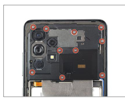
Use a Phillips screwdriver to remove the ten 4.4 mm-long screws securing the motherboard cover.
