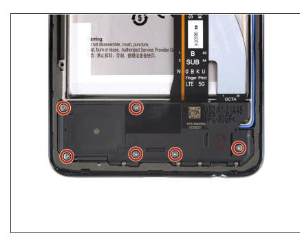
Use a Phillips screwdriver to remove the six 4.4 mm-long screws securing the loudspeaker assembly.
