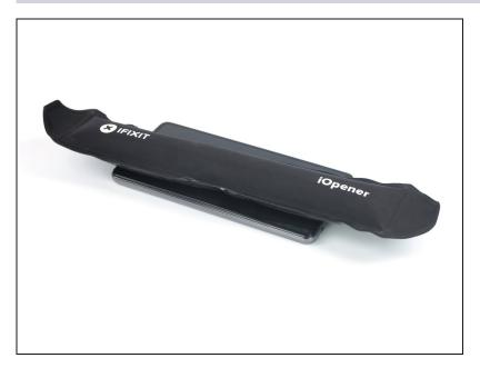
• Apply a <u>heated iOpener</u> or a heat gun to the screen to loosen the adhesive underneath. Apply the iOpener for at least two minutes.
