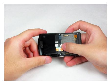
Remove the SIM card by pulling it toward the top of the phone with your thumb.
