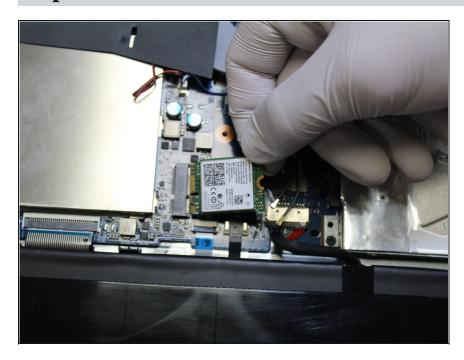
Pull the Wi-Fi card directly out of its port.
