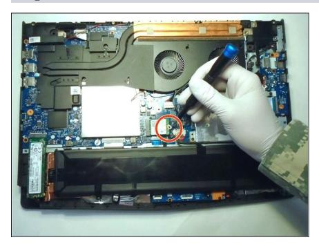
Use a Phillips #00 screwdriver to remove the single screw securing the Wi-Fi card.
