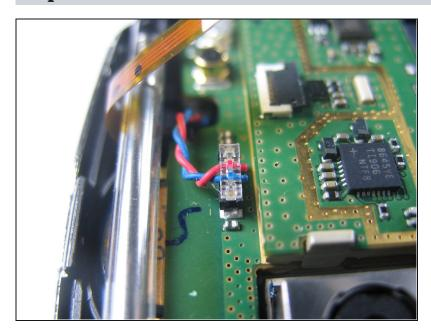
Remove the jack attached to the red and blue wires by carefully pulling it upward from the motherboard.
