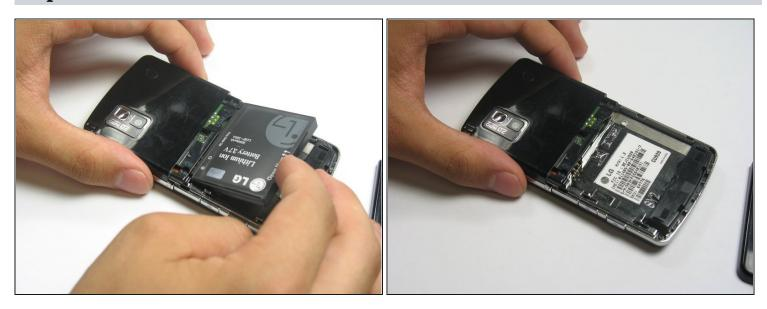
• Remove the battery by placing your fingernail or an opening tool at the bottom edge of the battery and lift it out.
