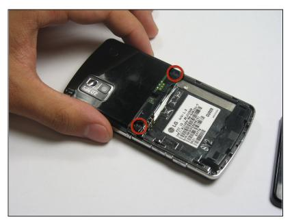
Remove the two 3.5 mm screws above the battery port with a Phillips #00 screwdriver.
