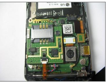
• Remove the plastic case to reveal the motherboard.
