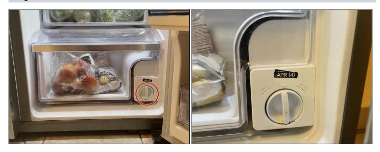
• Open the refrigerator door and locate the filter at the bottom right corner of the fridge.
