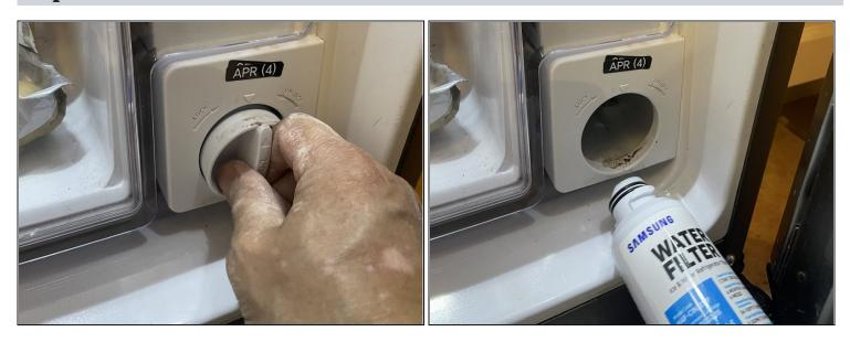
• Firmly pull the old water filter straight out to remove it.
