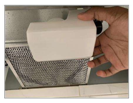
Squeeze both ends of the bulb cover to pop it out of the slots.
