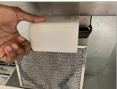
Reinsert the lightbulb cover by pressing both sides and fitting the cover's tabs into the slots.
