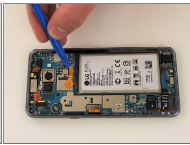
• Using an opening tool, carefully pry up the ribbon cable to disconnect the battery.
