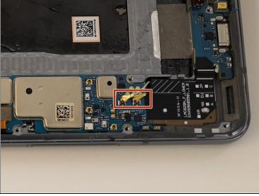
Use an opening tool to disconnect the two coaxial cables from the motherboard.
