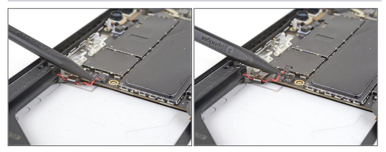
• Use the point of a spudger to lift the left speaker connector out of its socket on the motherboard.
