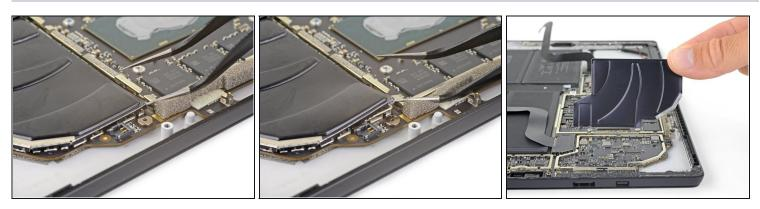
• Repeat the previous step to remove the remaining large EMI shield from the right side of the motherboard.
