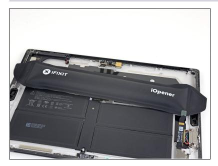
Heat an iOpener and apply it to the battery connector for two minutes to soften the adhesive securing the connector to the case.
