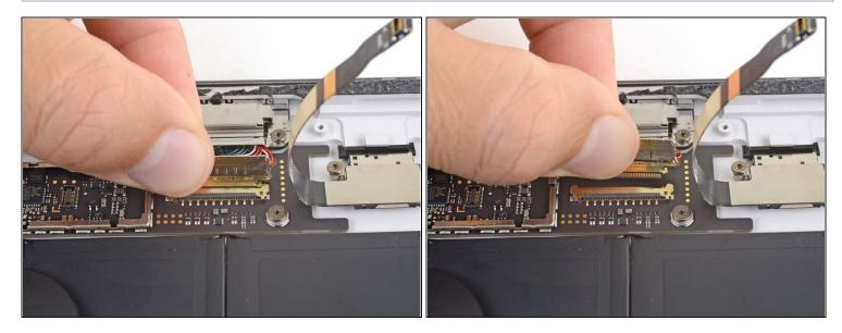
• Slide the SurfaceConnect port connector out of its socket on the motherboard.
