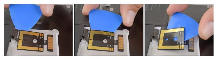
• Starting at the edge closest to the battery, slide an opening pick under the battery connector to separate the adhesive underneath.
