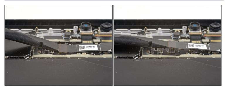
• Use the flat end of a spudger to pry the front-facing camera connector up and out of its socket on the motherboard.
