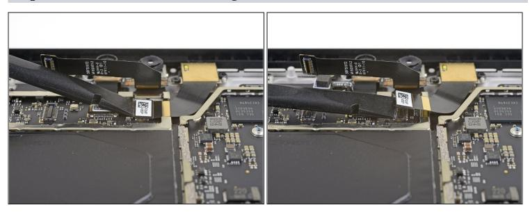
• Use the flat end of a spudger to pry the rear-facing camera connector up and out of its socket on the motherboard.
