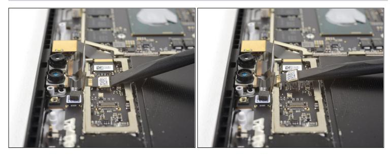
• Use the flat end of a spudger to pry the face-detection camera connector up and out of its socket on the motherboard.
