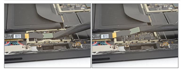
• Use the flat end of a spudger to pry the microSD card reader connector up and out of its socket on the motherboard.
