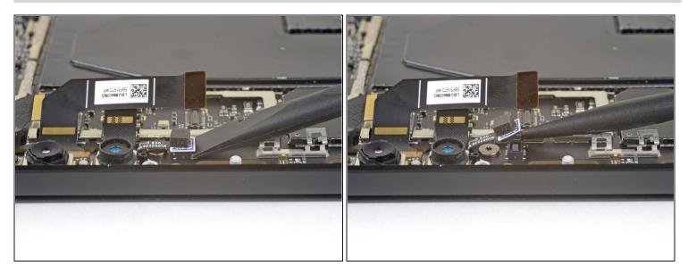
• Use the flat end of a spudger to pry the microphone connector up and out of its socket on the motherboard.
