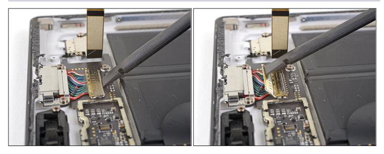
• Use the flat end of a spudger to lift the flap that sits over the SurfaceConnect port connector.
