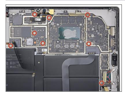
• Use a T3 Torx driver to remove the eight 2.5 mm screws securing the motherboard.
