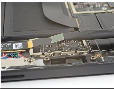
• Use the flat end of a spudger to pry the microSD card reader connector up and out of its socket on the motherboard.
