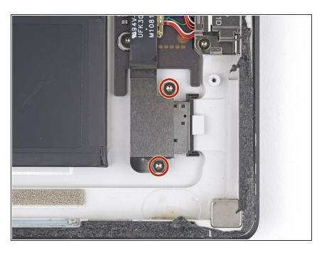
Use a T5 Torx driver to remove the two 3.1 mm screws securing the microSD card reader.
