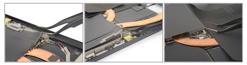
Repeat the last step for each corner of the EMI shield covering the heat sink.
