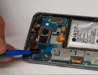
Using an opening tool, carefully disconnect the ribbon cables from both cameras.
