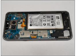
• Using an opening tool, carefully pry up and remove both cameras from the phone casing.
