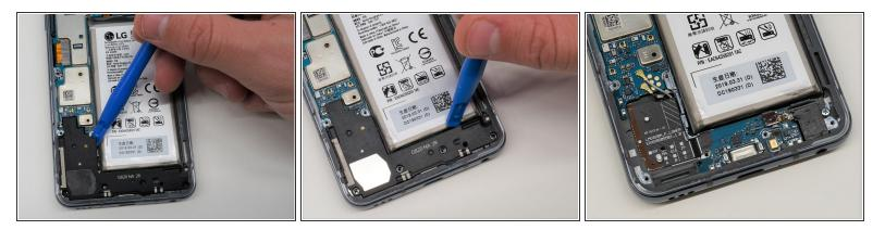
• Using an opening tool, carefully pry out remove the speaker system from the phone.
