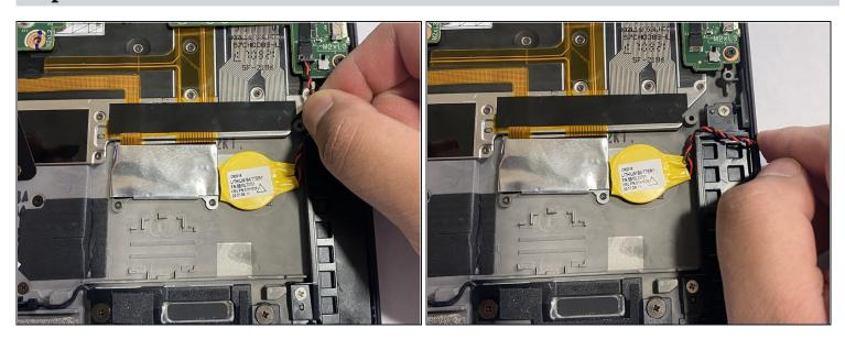
• Disconnect the CMOS cable from the socket on the motherboard.
