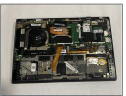
• Remove the battery using your hand or a prying tool.
