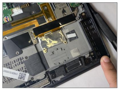
• Remove the CMOS battery.
