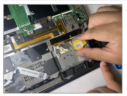
Once the battery is removed the CMOS battery will be exposed.
