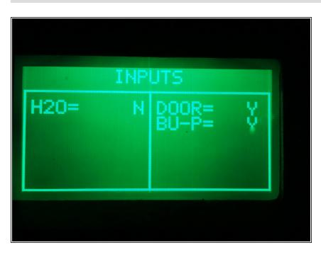
The sensors are displayed in the third menu. H20 stands for water tank, DOOR for the door sensor, BU-P indicates the brew group sensor. N means no, of course, Y means yes.
