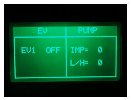
• The next screen is split. The electric valve can be seen on the left, closed here. Press the top left button to shift. On the right the pump or the impulses of the flowmeter. To test, press the top right button.
