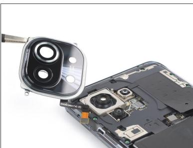
Use your fingers or a pair of tweezers to carefully lift the camera cover including the flash assembly off the camera lenses and remove it.
