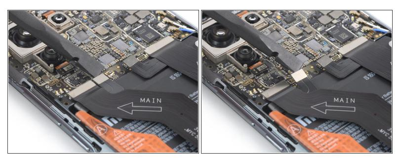
Use a spudger to disconnect the left battery cable by prying the connector straight up from its socket.
