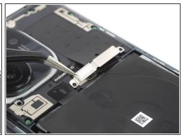
Use a pair of tweezers to remove the connector bracket by pulling it in the direction of the battery.
