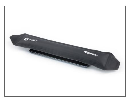
Apply a <u>heated iOpener</u> or a heat gun to the screen for two minutes to loosen the adhesive underneath.
