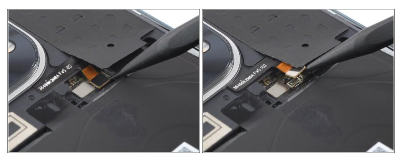
Use the pointed end of a spudger to disconnect the flash assembly cable by prying the connector straight up from its socket.
