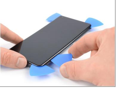
Insert a fifth opening pick and slide it along the right edge of the phone to slice the remaining adhesive.
