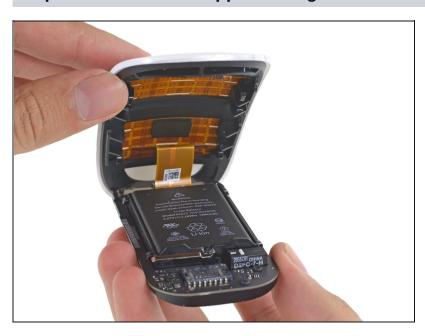
Open the battery compartment carefully. A ribbon cable connects the two halves.
