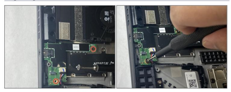
Use the Phillips #1 screwdriver to remove the two 1.2 mm screws.
