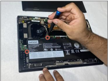
• Use the Phillips #1 screwdriver to remove the four 1.2 mm screws that secure the battery.
