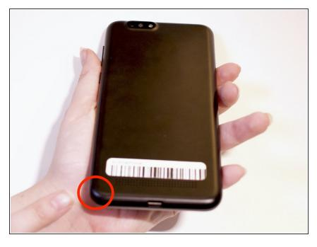
Using a fingernail pry open the back cover off with the bottom left indent.
