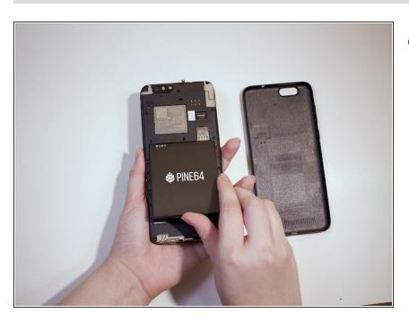
Using a fingernail, press into the bottom divot and remove the battery from the phone.
