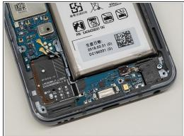
Using an opening tool, carefully pry out remove the speaker system from the phone.
