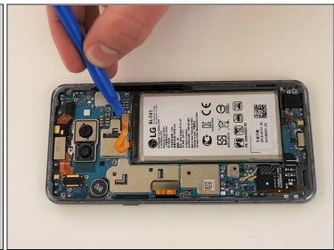
Using an opening tool, carefully pry up the ribbon cable to disconnect the battery.
