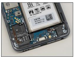
• Using an opening tool, carefully pry out remove the speaker system from the phone.
