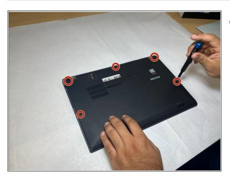
Use the Phillips #1 screwdriver to remove five 1.2 mm screws from the back cover of the laptop.
