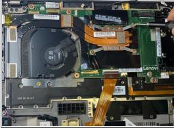
Use the Phillips #1 screwdriver to remove all five 1 mm screws holding the fan and heat sink down.
