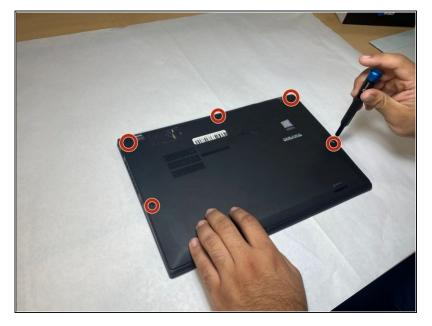
• Use the Phillips #1 screwdriver to remove five 1.2 mm screws from the back cover of the laptop.
