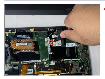
• Use the Phillips #1 screwdriver to remove the 1.2 mm screw that's holding the Wi-Fi card in place.
