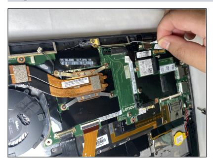
• Disconnect the white and black coaxial antenna cables from the Wi-Fi card.
